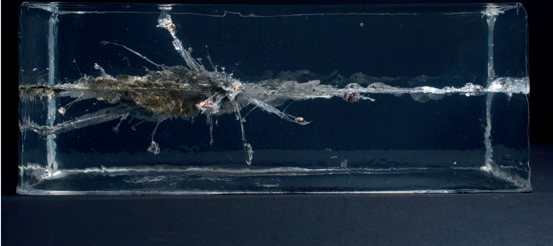
FRAGMENTS OF AK-47 AND M16 BULLETS FIRED AT ONE ANOTHER IN A BALLISTICS GEL BLOCK
